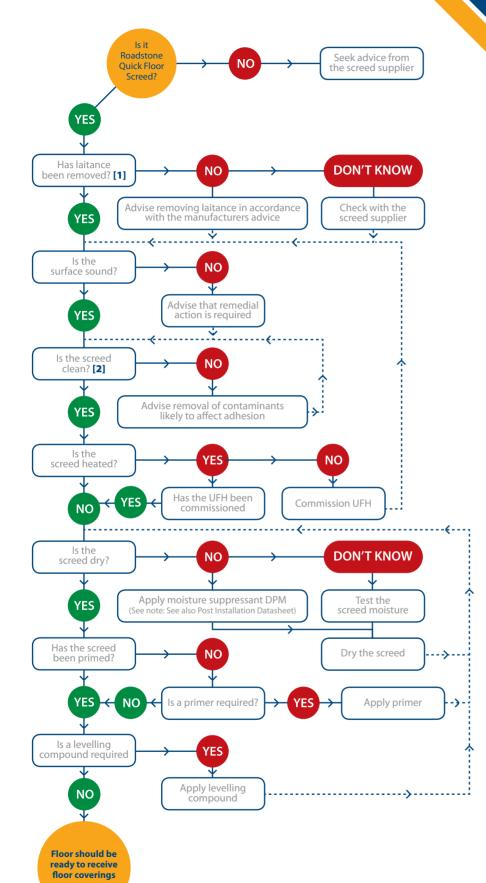
This datasheet is intended as a guide to the steps required with Roadstone Quick Floor Screeds in order to ensure that they are properly prepared to receive floor coverings. It may not cover all eventualities and should be used in conjunction with our other data sheets where appropriate and where manufacturers of other products are used the relevant manufacturers advice should be followed.
