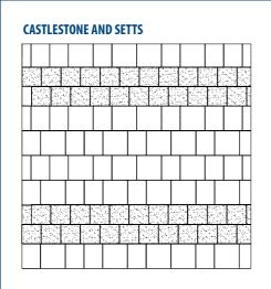
Indicative layouts shown represent a portion of a paved area but should not be used as a pattern to follow or continually repeat, as this may result in having a surplus of one particular size left over. Use all the paving sizes within each bale to cover the required paved area.
